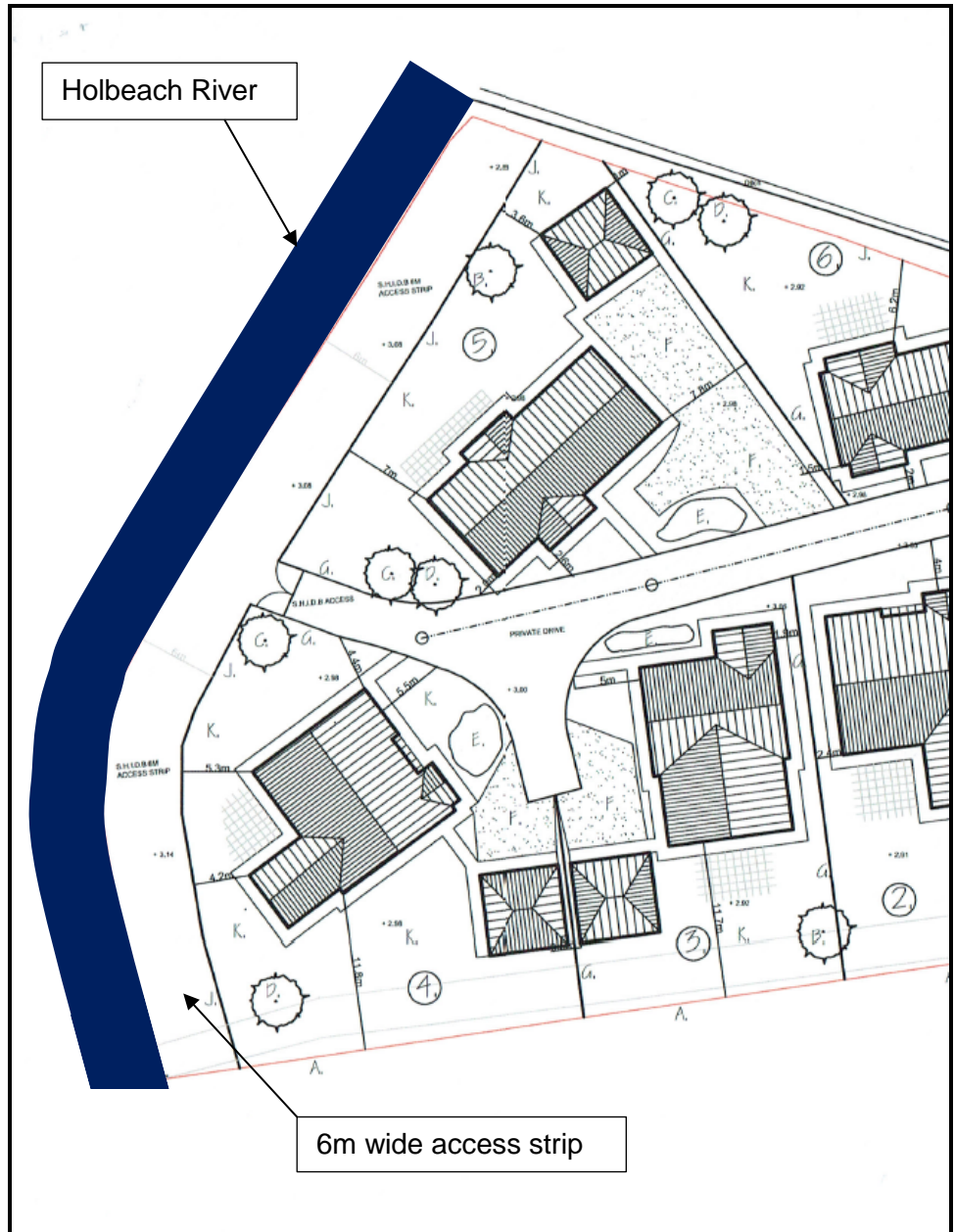
Detail of site plan showing 6m wide access strip
