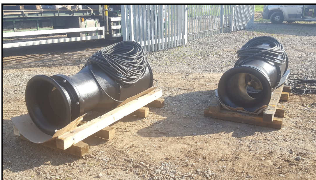
New fish friendly pumps prior to installation – May 2018
