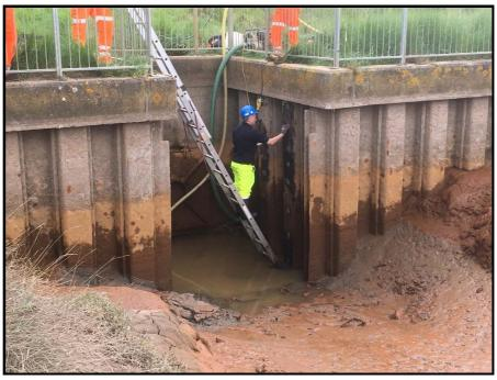
Fleet Haven Pumping Station outfall – Steel sheet piles prepared for ultra-sonic thickness testing, and the testing in progress
