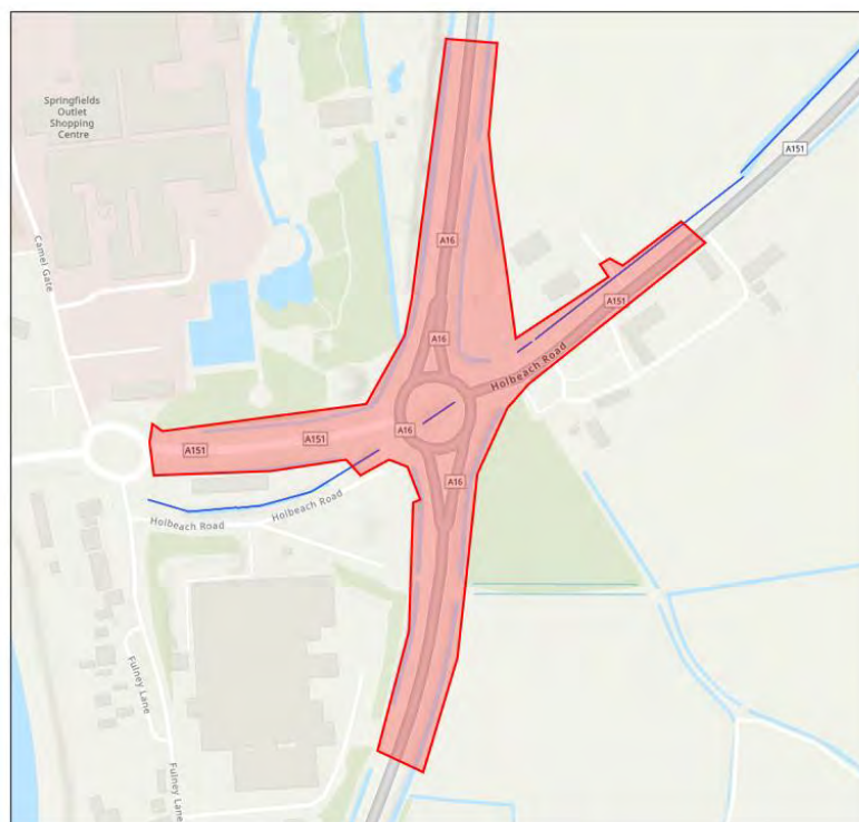
Figure 1: Roundabout improvement scheme extent, showing arterial watercourse within the existing roundabout centre.
