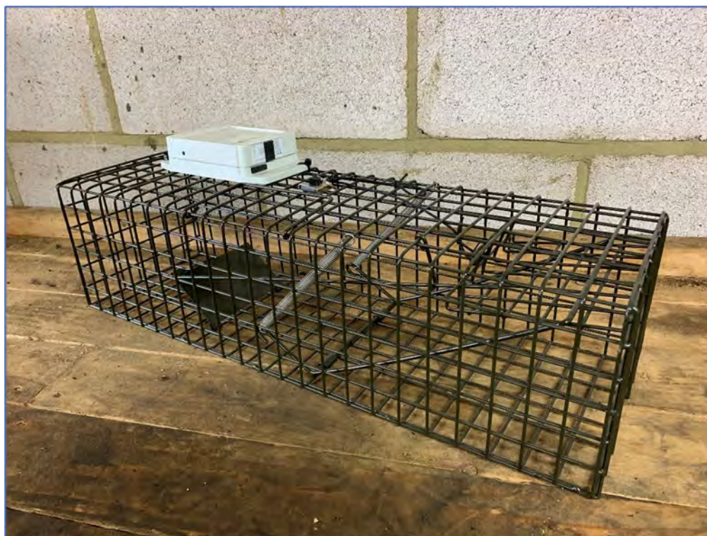
Remote Smart trap device connected to the trap which, when activated by the trap closure, will “text” the volunteer to inform them of a capture. This trap will be mounted in a floating raft to lure in and capture mink.
