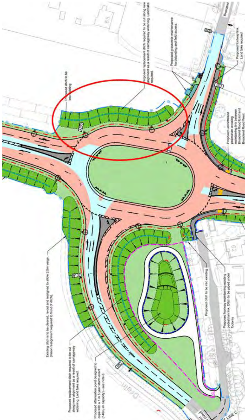
Figure 3: Extract of the General Arrangement. Drawing No. 5100975-SKA-HGN-BER2-DR-CH-0001 Rev. C01 (Cambridgeshire Highways, Aug 2020). Section of watercourse to be realigned and potentially abandoned circled with red line.
