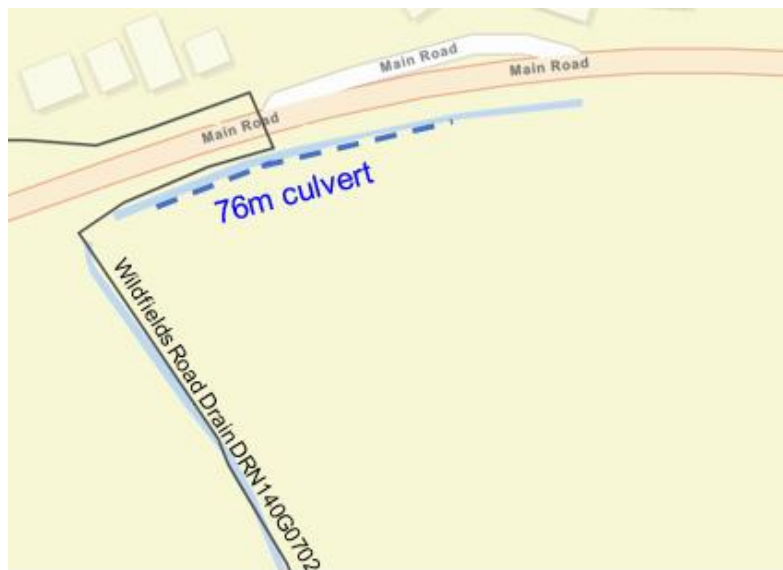
Figure 2: Location plan showing the proposed culvert location. The sections which are designated as Adopted Watercourses are shown using a solid black line.
