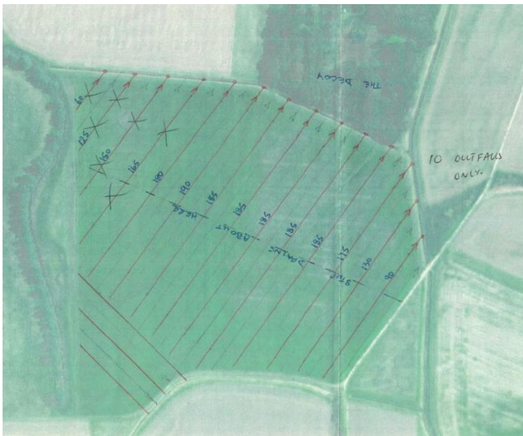
Figure 5: Proposed drainage scheme for site 2.
