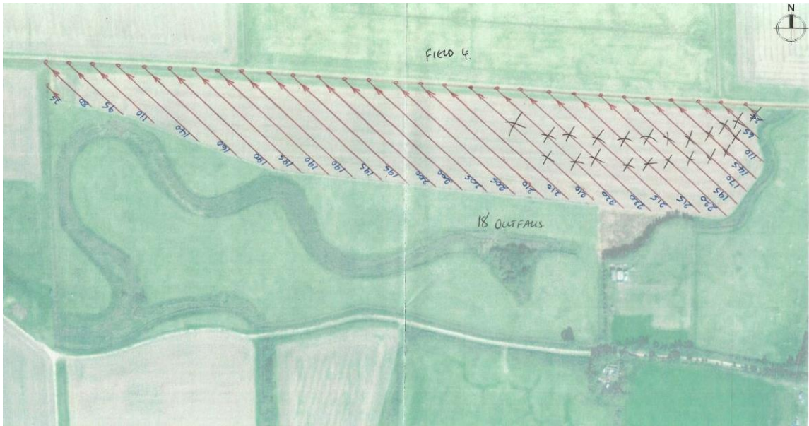
Figure 4: Proposed drainage scheme for site 1.
