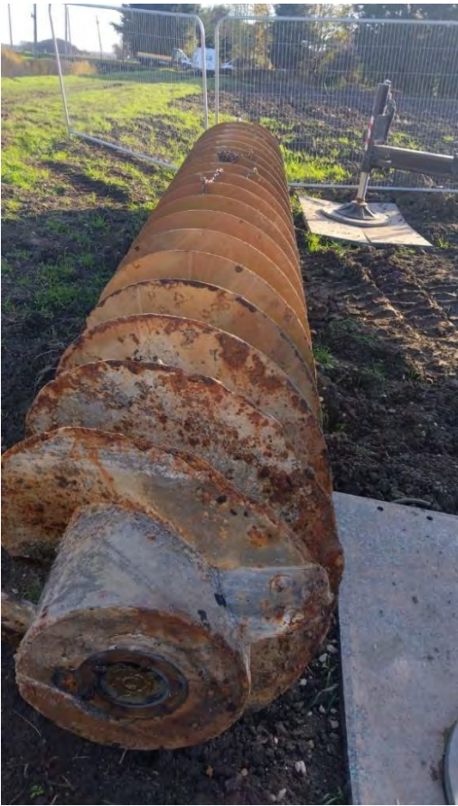
Heavily corroded old screw pump
