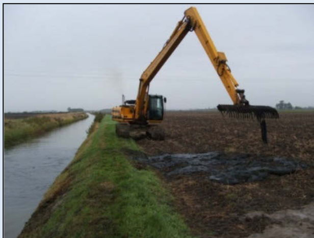
Excavator with 'cott rake' ©Witham Fourth District IDB
