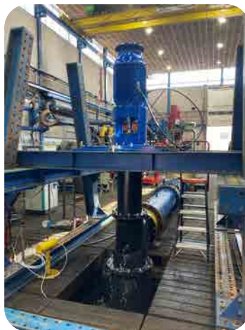
Factory testing of one of the new Horsey pumps & Horsey pumping station wet well in construction
